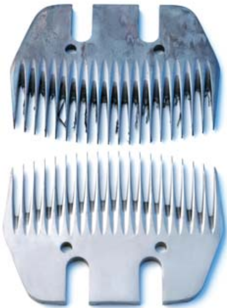
Carbon steel hair clipper blade untreated, FerroChem-treated
