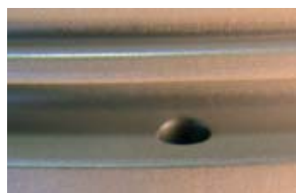
Drilled hole on a carbon steel ball bearing race before and after FerroChem-treated
