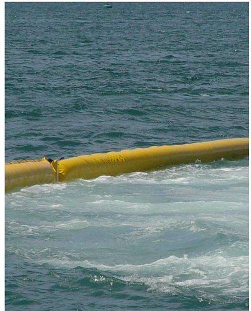
Examples of an oil boom operation by means of an inflatable oil boom
