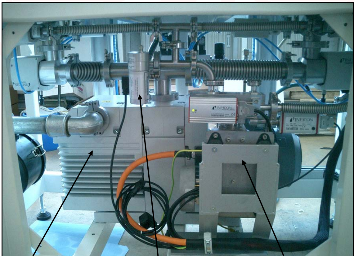
Vacuum Pump module
